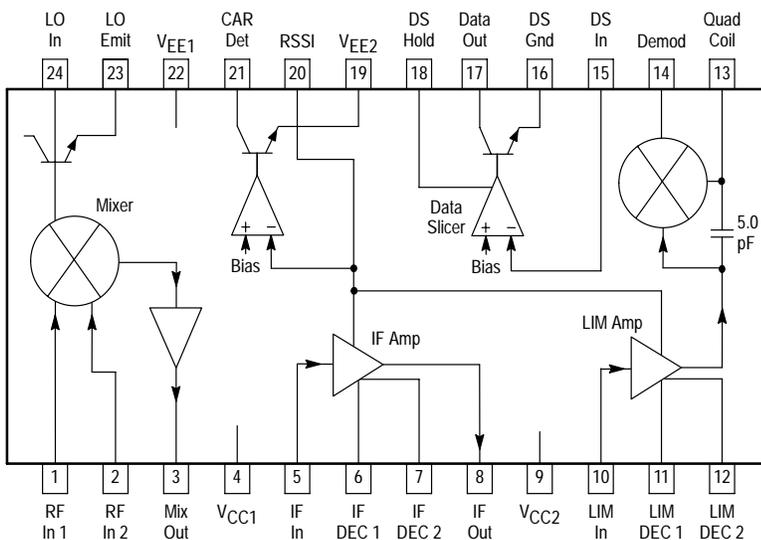
NOTE: Pin Numbers shown for SOIC package only. Refer to Pin Assignments Table.
