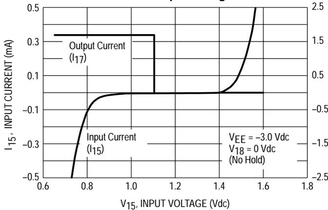
Figure 16. Data Slicer Input Current versus Input Voltage
